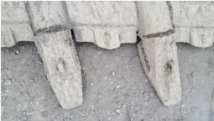
Figure 3: Loader teeth which must be changed periodically.
