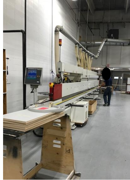
Figure 2: Monitoring material while running through edgebanding
