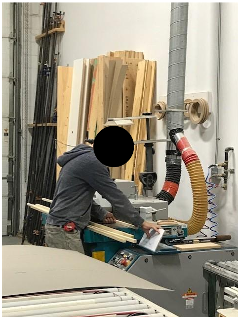
Figure 3: Use of the shaper to trim materials
