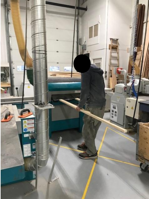
Figure 3: Use of the shaper to trim materials
