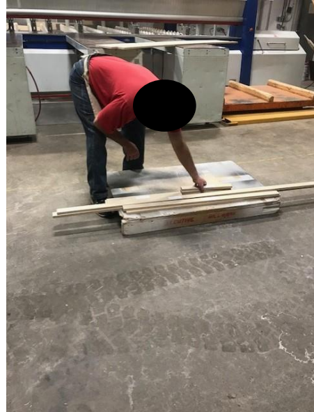
Figure 6: Placing cut materials on pallets
