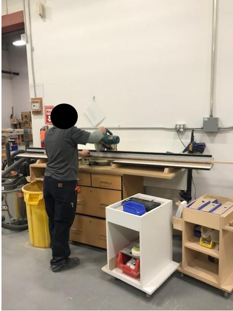
Figure 5: Using chop saw to cut base supports
