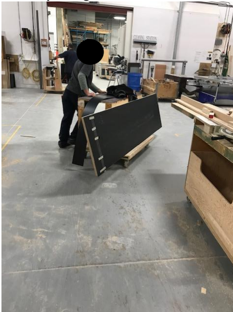
Figure 7: Transporting materials with vertical cart
