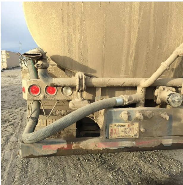
Figure 3: Hose attachment at the back of water truck and where the water sprays out.
