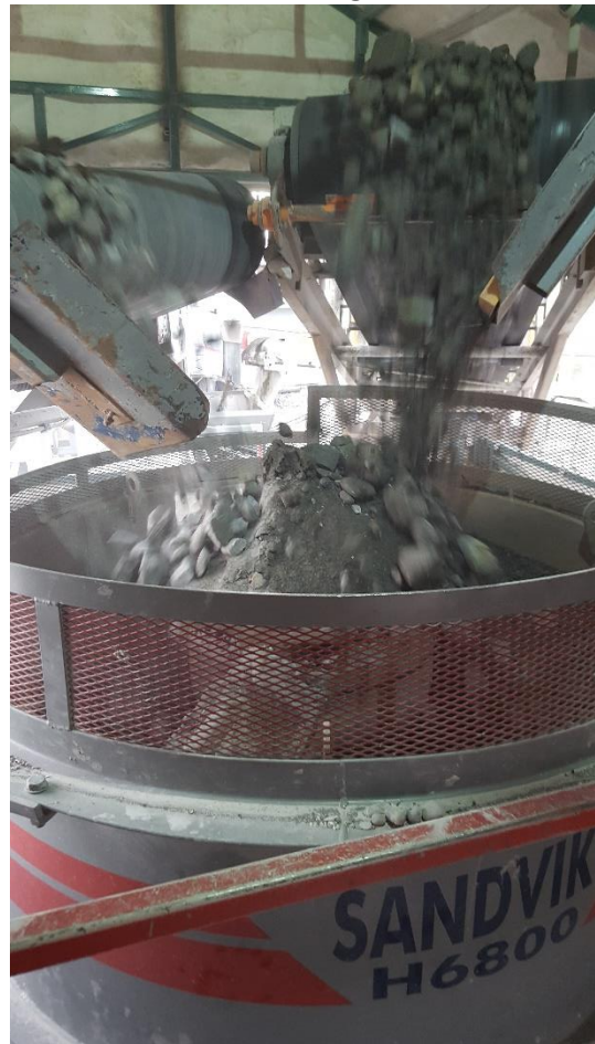
Figure 4: Cone head which requires regular maintenance and cleaning.
