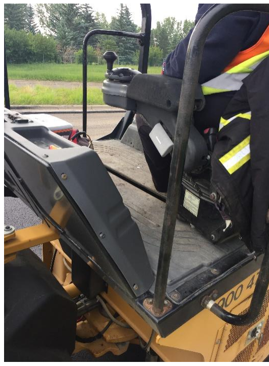
Figure 4: Left side controls of Steel Drum Roller.
