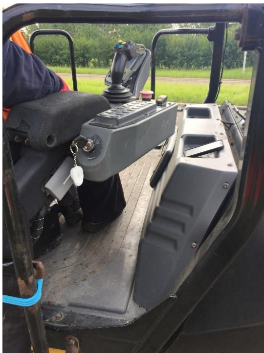
Figure 3: Right side controls of Steel Drum Roller.
